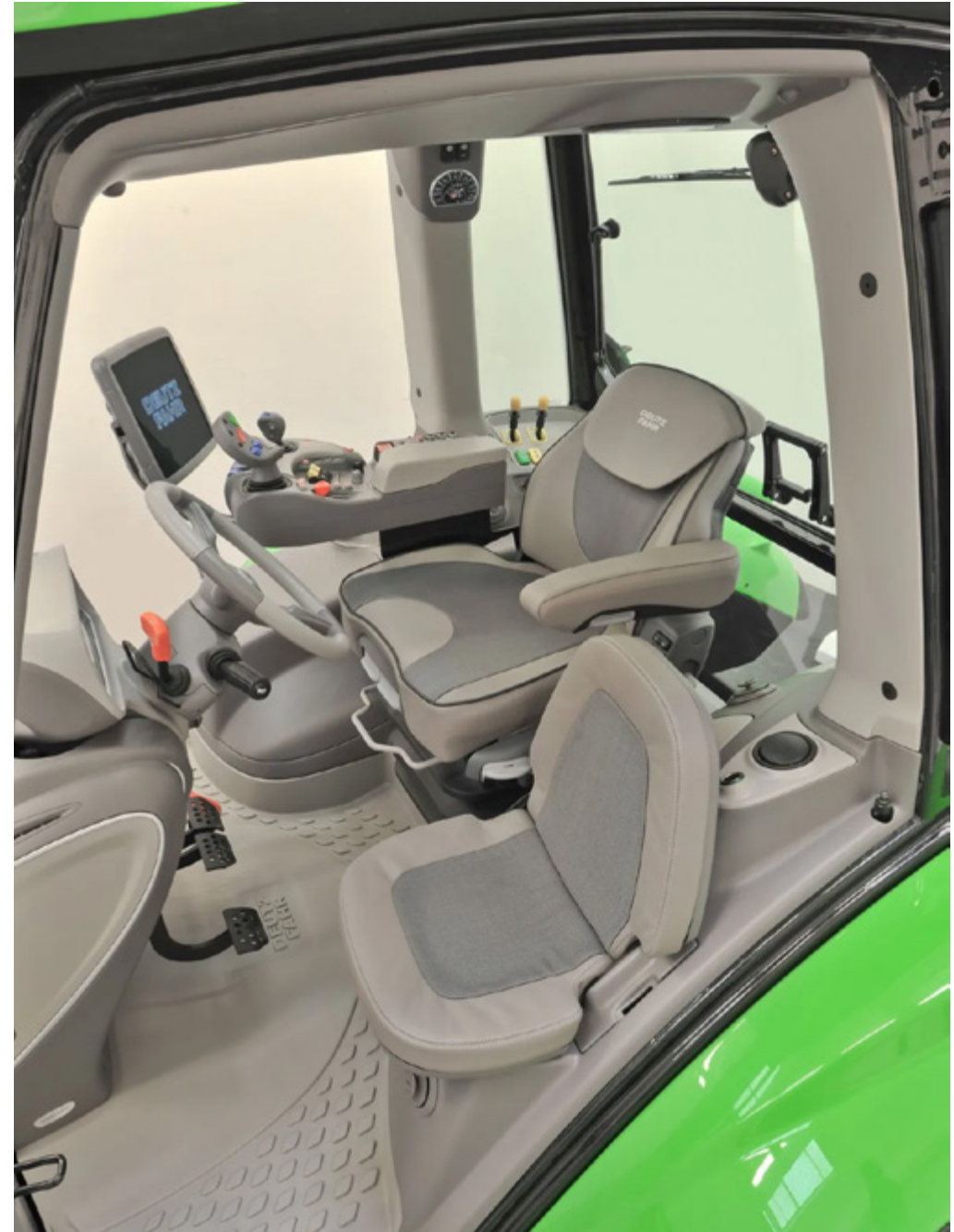
> The revamped MaxiVision 2 Cab sets a new benchmark in its class, thanks to air suspension, high-quality materials, great roominess and careful control design.
