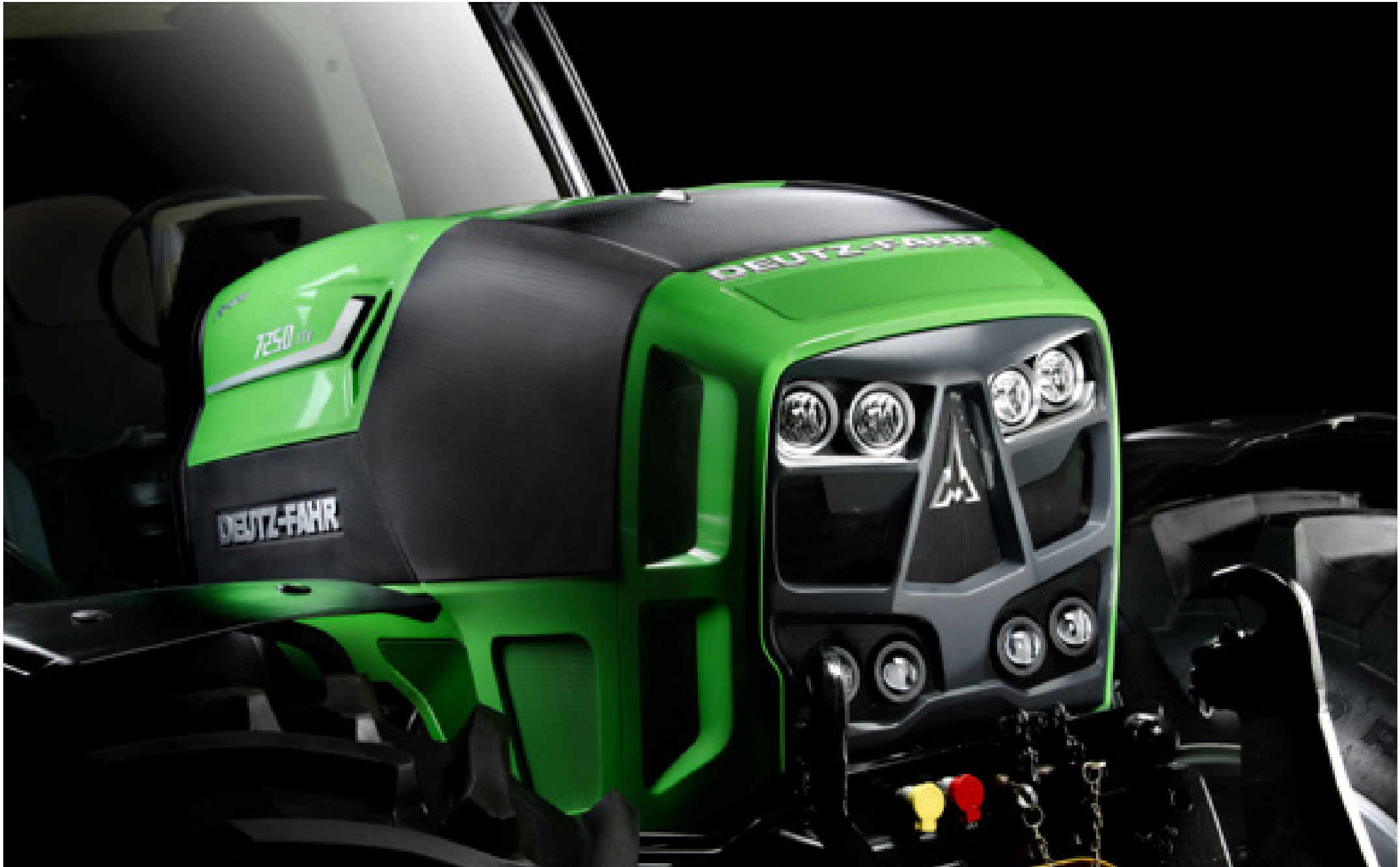
> The front of the tractor features a moulded bonnet that integrates the headlights and provides stress resistance.
