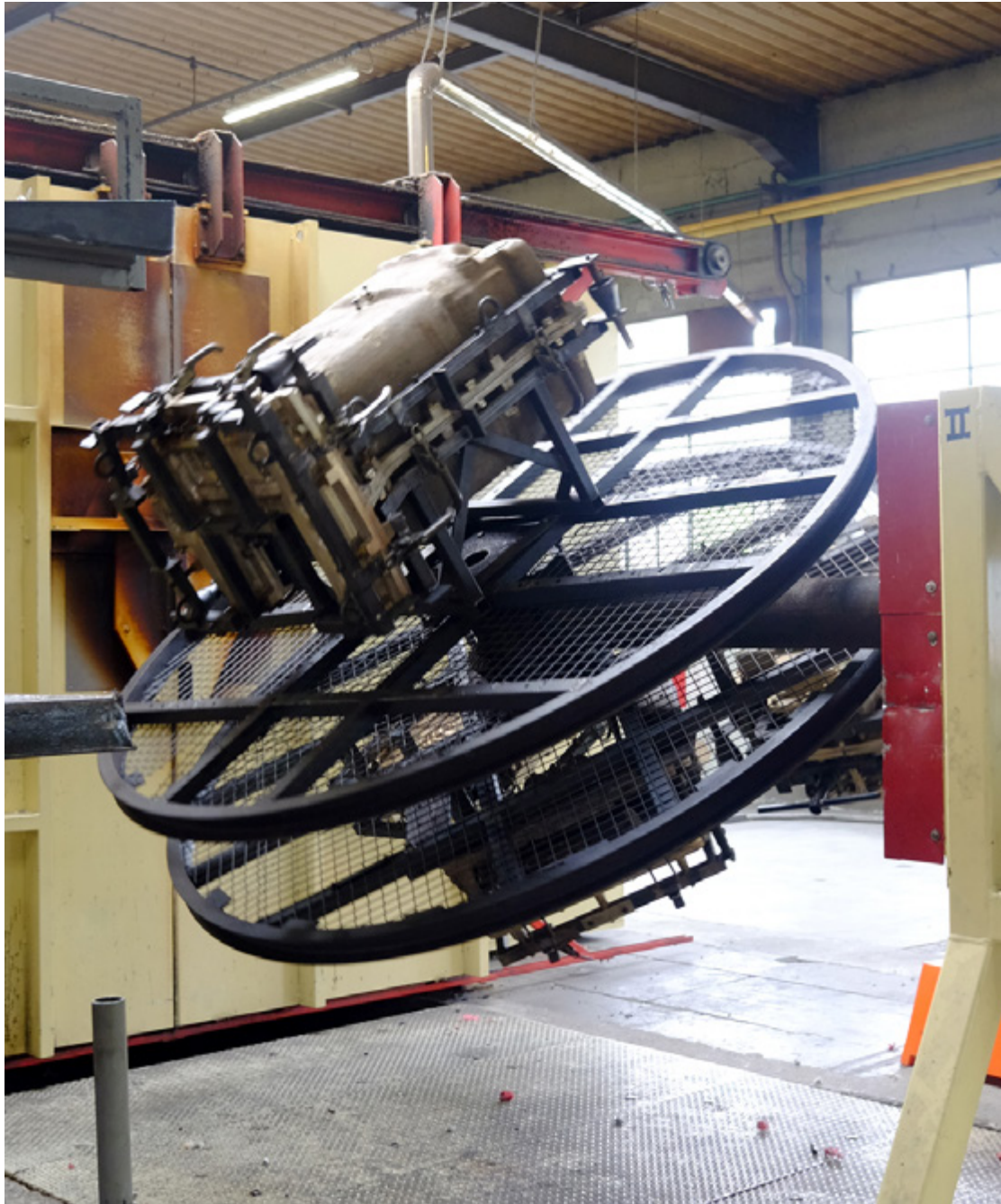
> The structure is rotationally moulded and integrates a series of accessory elements such as rear wheels.
